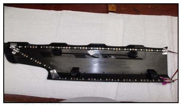
This shows the position of the led strips on the passenger side cover. Always use degreaser and alcohol swabs to clean the mounting area. Use the same procedure to mount all the strips in the correct position. Secure the wires with the supplied heat duct tape.
