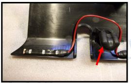
Test fit the strips so you have a good idea how they will fit. Start here and route the wire behind or under the large retaining hook. Remove the backing from the strip and press in place. The backing is easier to remove if you score it with a razor blade as shown. Use caution and don't cut too deep. Use the large picture above to trial fit and mount all the strips. Now use the supplied heat ducting tape to secure the wires.
