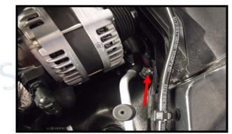
The long black wire has to be routed up to the ground stud located ahead and below the alternator. Secure the black wire with the provided nut and tighten. Now hide and secure all wires and use the supplied cable ties to secure them. Always re check wires and strips after a while to be sure they are all secure. You can install 1/4" wire loom over any exposed wires to hide them better.
