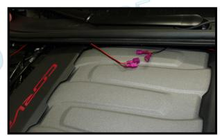
Connect the coil cover wires together, red to red and black to black. Drop the wires down behind the engine to hide them.
