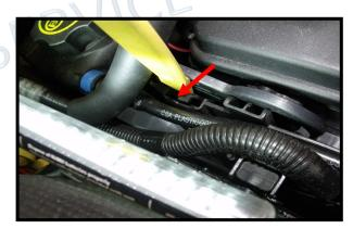
To gain easier access to the positive connection point you can raise the large handle out of the way by releasing the locking tab on each side of the fuse box and pulling it up. .
