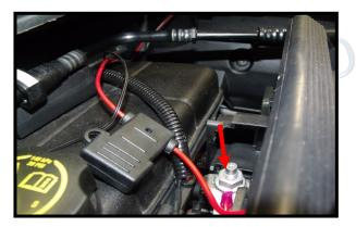
If installing a switched kit, route the wires toward the large terminal at the back of the under hood fuse box. If mounting a remote control kit, forward to that section.
