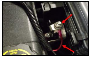
Remove the 13mm nut and connect the fused red wire. Point the red wire so it follows the factory cable so you can close the cover.
