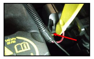
Pry this tab back and flip up the cover over the positive terminal at the back of the fuse box.
