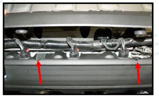
Install the coil covers by aligning the retaining hooks with the V shaped area indicated by the red arrows. Once fully in place you can just push down on the side opposite the hooks to click them in place. Be sure they are secure.
