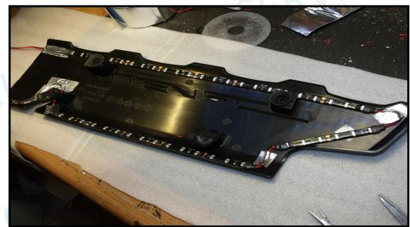
This shows the drivers side location of the led strips. First, wipe down the mounting area with degreaser then alcohol swabs. Next, cut the very top off the adhesion promotor pack. Squeeze the excess fluid back into the packet as you remove the sponge. Apply a thin coat to the area where the strips mount. Let dry for a 2 minutes. Apply the strips within 1 hr.
