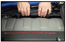
Remove both fuel rail covers by pulling up as shown. Then slide them towards the center of the engine then remove.
