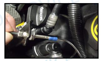
Slide the switch through the hole, start the nut then plug the black wire into the bottom before tightening the nut. Hold the top nut with the 7/16" wrench and tighten the bottom nut with the 9/16" wrench. It is a nylock nut so it will be hard to tighten but it wont come loose! The leds should now lite. Test the switch operation by closing the hood and observing if the lights go off. If not you can raise the switch by placing a 3/8" washer under the top nut.
