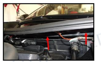
After mounting the led strips and the coil covers back on the car, route the wires and control box up under the cowl and attach with provided tape. You can mount the box under the cowl lip or on top of the coolant reservoir. Connect the red fused wire as directed in the switched kit instructions.
