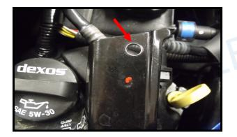
The red dot shows where the hood bumper hits so do not drill the hole there. Drill a 3/8" hole as shown. Put a towel under this area to catch the filings. Be careful to not drillinto things under this brace. If yours is a Z51 car be careful of the lines under this bracket.
