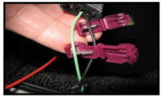
Strip back the wire covering so you can install the supplied connectors. Make sure the connectors are at least 2 inches away from housing to allow re-installation of the housing. Place each wire into the metal clip and fold the clip closed until it clicks shut. You may have to use a pair of pliers.
