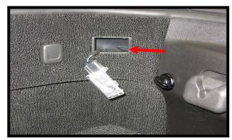
Remove either rear hatch light housing by prying it out at the inner edge. (red arrow).
