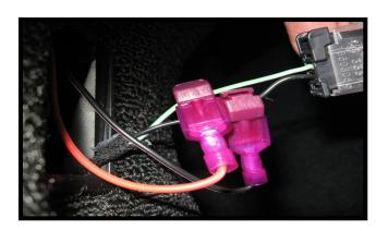
Now plug the led strip leads into the back of the connectors as shown. Red connects to the green wire and black to black. LEDs should now light up. If not, make sure the interior lights have not timed out which they will do after about 15 minutes. Open and close the door or start the car to reset.
