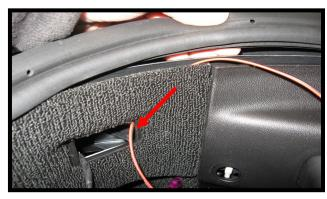
Pull up on the weather strip so you can route LED wires behind the panel and through the light opening. (red arrow).
