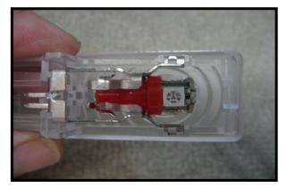
Install the led into the light housing. If it doesn't light, remove it turn it 180 degrees and re-install it. Also make sure the lights haven't timed out which they will do after about 15 minutes.
