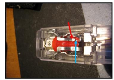
If you are still having trouble getting it to light make sure the factory contact (red arrow) is contacting the small led wire (blue arrow). If they are not contacting each other you can move one or both of them to get contact. After all is working re-install the housings and enjoy the new lights!
