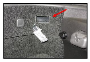
Start by prying the factory light housing out of the panel at the inside edge of the housing (red arrow).
