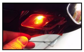
Enough tinting is supplied to do both sides twice in case you make mistakes. Remove the adhesive backing by biting a corner of the film with your teeth and separating it. Carefully lay the film over the light making sure the entire light is covered.
