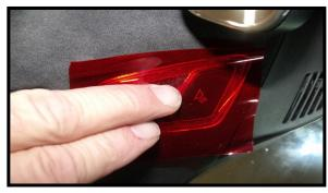
Start in the middle of the lens and work the film out toward the edges making sure to eliminate bubbles and wrinkles. It helps to lift the film with one hand and press the film outward with the other .
