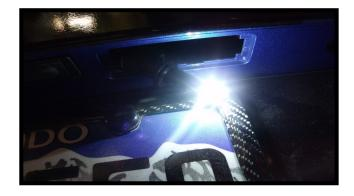
Turn on the running lights. Insert the led. If it doesn't light turn it 180 degrees and re-insert it. Use the same procedure for both license plate bulbs.
