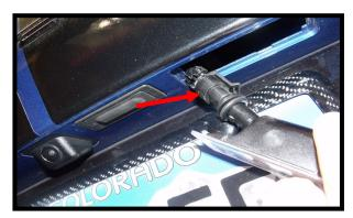
Hold the black connector then turn the housing counterclockwise and remove the factory bulb. It may be hot!
