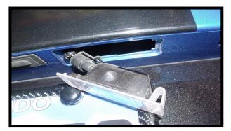
Insert the socket into the housing by aligning the tabs. Then turn the housing clockwise to lock it in place. Place the housing back into the opening clipping the right side in first then the left.
