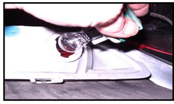
Remove and unplug the factory bulb. It pulls straight out of its socket.
