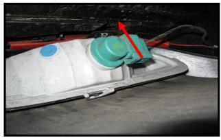
Unlock the reverse light connector by turning it 1/4 turn upward or counter clockwise. Take note of the position of the socket when it comes out . You will need to line up the tabs on the socket with the slots in the housing and turn it 1/4 turn down or clockwise.
