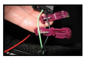
About 8" or so from the socket, strip back some of the covering to gain access to the brown and black wires. Using the supplied quick tap connectors, place the factory wire in the metal clip as shown and fold it closed until it snaps shut. Do this for both wires on each side. You may need to use pliers for this. Note: The wires you will see will be brown and black.
