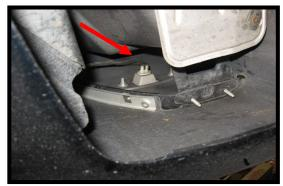
You need to gain access to the rear side marker bulb to do the wiring. Depending on what exhaust system you have you may be able to reach up from underneath to remove the bulb socket by twisting it 1/4 counter clock wise. If you can't access it that way you can remove the outer taillight on each side to gain access to the wiring.
