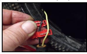
Reach through the tail light opening and locate the upper brake light. Unlatch the connector and pull out so you can tap into the wires. Twist the ends of the red led wires together, same with the black. Crimp the spade terminals on the red and black wires. Using the supplied quick tap connectors tap into the yellow and black wires. Plug the red LED wire into the yellow wire and the black to the black. Step on the brakes to test the lights.
