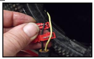
If you haven't done so remove the outer tail lights. Unlock and unplug one of the tail lights. Using the supplied quick tap connectors, tap into the turn signal positive wire. LR: Yellow, RR: Green. Tap into the black negative wire on both sides, Plug the LED red wire into the positive wires, yellow OR green, and plug the LED black wire into the black factory wire. See last picture on 1st page to see how connectors plug into the quick taps. Test lights before re-installing tail lights.
