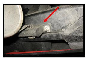
Locate the muffler hangar. (red arrow). The led bar will mount directly behind the hangar facing the rear of the car. Don't mount the bars yet. When you do mount the led bars remember the wires go to the outside of the car
