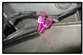
This shows both wires with the quick connectors installed and the led wires plugged in to the back of the connectors. Connect the black led wire to the black factory wire. Connect the red led wire to the brown factory wire. Make sure the connectors are fully seated against the quick tap. Now you can test the leds by turning on the lights.
