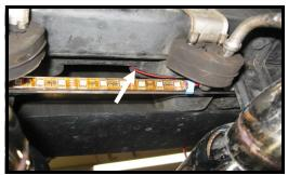
This shows the location of the exhaust leds. Led bar is attached to the rear of the rear facia brackets facing the front of the vehicle. Note the routing of the wires. (white arrow) going up towards the license plate lights. This is where the wire hangar comes in handy.
