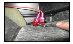
Strip back some of the tape holding the wires together to give room for the quick taps. Center the wire in the foldable connector and close it together with pliers until it locks in place. Connect the led wires into the back of the connectors. Black to the black wire and red wire to the dark brown wire. Push leads in firmly until they bottom out on the connector as in this picture.
