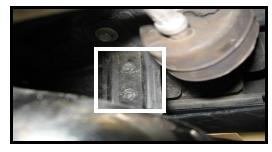
This shows the rear facia bracket that the led bar attaches to on the back side between these 2 screws. Leds face the front of the car. Center the bar between the brackets, peel and stick the led bar to the backside of the brackets between the screws.
