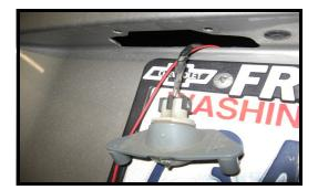
Remove 2 screws that hold one of the license plate lights in place. Using the coat hangar, route the hangar from the exhaust plate up to the license plate light. Tape the end of the led wires to the hangar and pull it up to the license plate light as in this picture.
