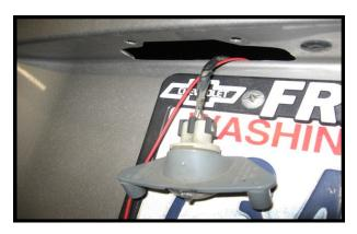
Use a # 15 torx bit to remove one of the license plate Housings. Peel back some of the covering on the wires so you can install the t-taps. Place one wire in the metal V of the t-tap and snap shut with a pair of piers. Repeat for both wires.
