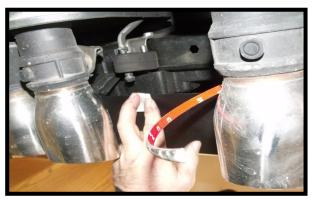
Wipe the rear edge of the rear fascia above the tailpipes where the leds will be mounted with the alcohol pad.
