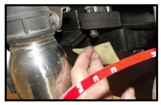
Cut the very top off the adhesion promoter pack and squeeze the excess fluid back into the packet. Fold the top over and seal to preserve the fluid for other kits you may have purchased. Wipe a thin coat on the mounting area of the car and let dry.
