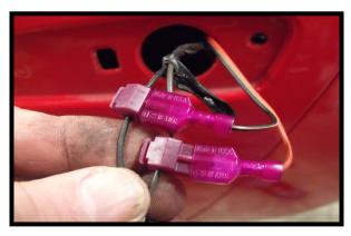
Fish the red and black led wires up through the license light opening keeping wires away from the exhaust and plug the red wire into the brown wire connector and the black to the black as shown. Turn on the lights to test.
