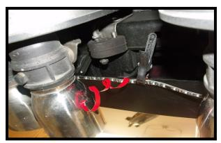
Center the led strip over the exhaust and peel the red backing from the strip. Mount the led strip to the rear edge of the rear fascia as shown. Press and hold in place for a minute or two.
