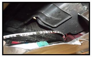
Now drop the led strip down behind the trunk/hatch area to the tailpipe area.
