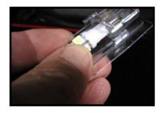
Install the led bulb into light housing. If it doesn't light, remove and turn it 180 degrees and re-install. It should now light. Make sure the interior lights havent timed out which they will do every few minutes. Re-install light housing
