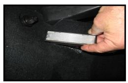
Pull the hatch/trunk light housing from the carpet to gain access to the back of the housing.
