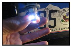
The bulb may be hot so use a shop towel to grab it and Turn on the lights. Plug in the led bulb. If it doesn't light, turn it 180 degrees and re-insert. Once the leds are working reverse the above steps to reinstall the light housings.
