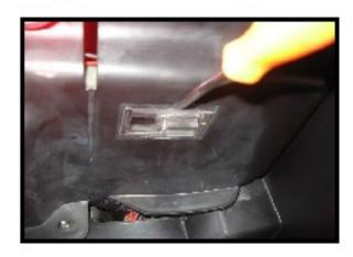
Using a flat blade screwdriver, carefully pry the footwell light housing out of the panel. Remove the factory bulb. DO NOT USE METAL OBJECTS TO REMOVE BULB TO AVOID BLOWING FUSE. Bulb may be hot.
