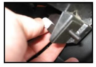
Open the glove box and remove stock bulb from housing. Bulb may be hot. Install LED into housing. If it doesn't lite, turn it 180 degrees and re-install. Bulb should not lite.
