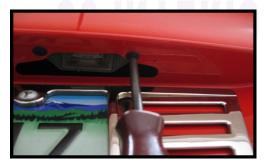
Using a #15 Torx screwdriver, remove the 2 screws holding the license light in place.
