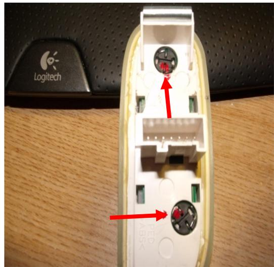
This shows the passenger side leds after they have been turned 1/8 turn into position. Top led in the 6 o'clock position and the bottom one in the 9 o'clock position. Plug the switch in and test the leds. Hook the bottom of the switch into the door panel and snap switch back into place.
