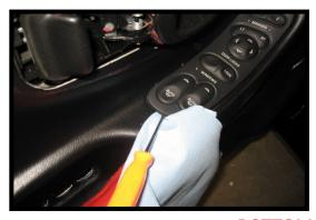
Remove drivers side window switch panel by prying up on the **BOTTOM** of the panel as shown. Remove the passenger side by prying up on the **TOP** OF THE PANEL. You will see 4 small sockets on the drivers side and 2 on the passenger side. Simply turn them 1/8 turn counter clockwise and remove all 6 factory bulbs. Refer to the diagram below for installing the LEDs.
