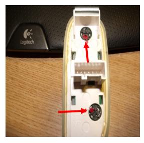
This shows the passenger side leds after they have been turned 1/8 turn into position. Top led in the 6 oclock position and the bottom one in the 9 clock position. Plug the switch in and test the leds. Hook the bottom of the switch into the door panel and snap switch back into place.
