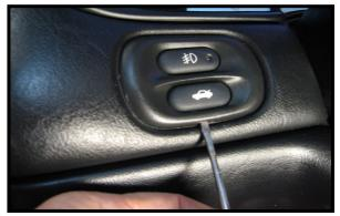
Locate the slot in the bottom of the hatch/fog housing. Using a small screwdriver pry the housing from the dash.
