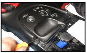
Open center console. Using a small pry tool pry the A/H Panel up and out of the console. Disconnect the wiring harnes. fitting flat screwdriver, turn the bulb counterclockwise 1/4
