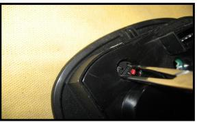
Using the same procedure as on the hatch switch, install the leds and twist them into place. Turn on the lights and plug the panel in to test. If they don't light remove the led, turn it 180 degrees re-install.
