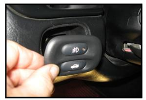
Re-connect the wire harness and press the switch back into the dash.
