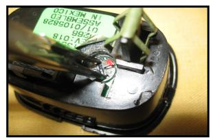
Insert the led by lining up the hooks on the leds with the slots on the back of the switch. Twist 1/4 turn clockwise to lock them in. If the leds are very tight you can first use a small file or dremmel to enlarge the hole very slightly. You can use a tight fitting screwdriver or a pair of hemostats and twist them in. Turn on the lights to test. If they don't light remove them and re-install them 180 degrees
