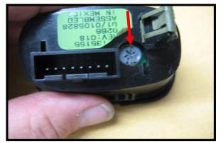
Red arrow shows the location of the bulb that needs to be changed. With a flat screwdriver, turn the bulb socket 1/4 turn counter clockwise and remove the bulb.
