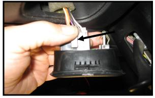
Depress the release tab and disconnect the wiring harness.
