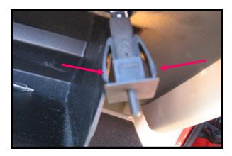
Open the glove box and locate this switch that holds the bulb. The red arrows show the 2 tabs on the back of the switch that need to be squeezed together to remove the switch. You can also disconnect the switch to make it easier. Remove factory bulb and insert led bulb. If it doesn't lite, turn 180 degrees and re-install. Re-connect the switch and re-install the switch in the panel.
