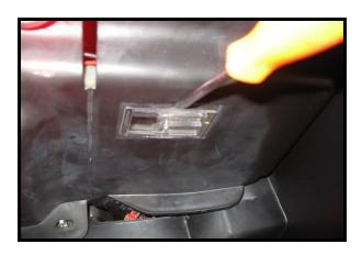
Using a flat blade screwdriver, carefully pry the footwell light housing out of the panel. Remove the factory bulb. DO NOT USE METAL OBJECTS TO REMOVE BULB TO AVOID BLOWING FUSE. Bulb may be hot.
