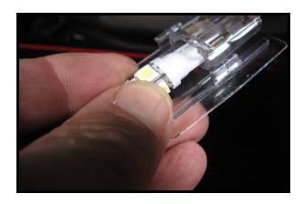
Install the led bulb into light housing. If it doesn't light, remove and turn it 180 degrees and re-install. It should now light. Make sure the interior lights havent timed out which they will do every few minutes. Re-install light housing
