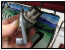
Remove the light housings, twist the grey socket 1/4 turn counterclockwise to remove it from the housing.
