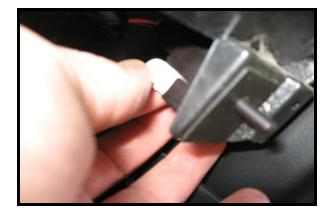
Open the glove box and remove stock bulb from housing. Bulb may be hot. Install LED into housing. If it doesn't lite, turn it 180 degrees and re-install. Bulb should not lite.
