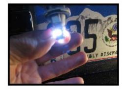
Turn on the lights. Plug in the led bulb. If it doesn't light, turn it 180 degrees and re-insert.
