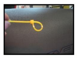
Remove the factory bulbs. (careful, they may still be hot). A little trick we like to use is using a small plastic wire tie to slip around the base of the bulb, pull it tight and pull the bulb out. Avoid using anything metal to remove them as you may short out the contacts.
