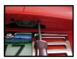
Using a #15 Torx screwdriver, remove the 2 screws holding the license light in place.
