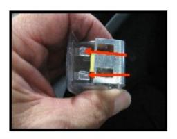
Remove the bulb shield by un-latching it from these 2 plastic tabs.
