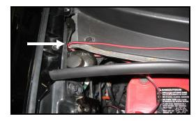
Pass the wire behind the rubber hood stop on the passenger side and so you can route the wires by the battery.
