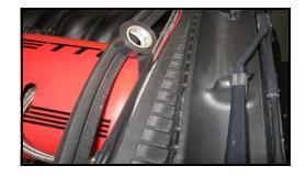
You can now test the cove lights. Make sure they are working before re-assembling. Secure the wire across the cowl with black electrical tape before re-installing the weather strip. Make sure not to pinch the wires. Attach control box if you havent already done so.
