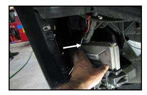
white arrow shows about where the white hangar may come through. Tape the led strip to the other end of the coat hangar and gently pull it through.
