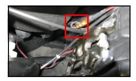
Thread the drivers side led strip through the hood cable loop behind the hood latch. This will drop the leds into the cove area.
