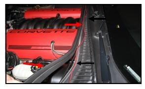
Lay out the harness with the controll box by the battery and string out the long wire across the cowl over to the drivers side. (black arrows) Remove the cowl weather strip. (red arrows).
