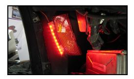
Wipe the mounting area with the provided alcohol pads. Peel and stick the strips near the cove opening pointing toward the inside of the car. You can also experiment with mounting the strips on the cove shield if you want them to shine out of the opening more.
