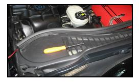
This shows the wire secured under the cowl strip. Always test the lights after the wiring is completed.
