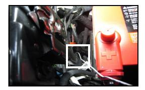
This is where a coat hangar comes in handy. Use the hangar to find a path for the led strip to get into the cove area.
