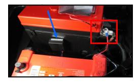
Remove the cover over the battery terminal on the under hood fuse box. (red box). Attach red wire from controll box using the supplied large washer and nut. Tighten. Blue arrow shows where the control box can be mounted once all wiring is secured.
