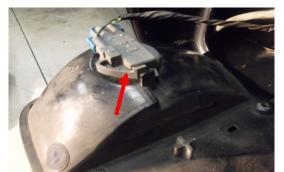
Cover the area below the housing before you lay it down to protect your paint. Press the locking tang in and turn the socket i/4 turn counter clockwise. Remove the bulbs by pressing them in and turn 1/8 turn counter clockwise.
