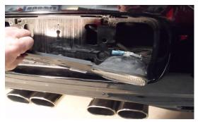
Now line up the socket with the slots in the housing and install. Lock it in place by turning it 1/4 turn clockwise.
