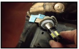
Line up the pins on the led housing with the channels in the socket. Push it down and turn it 1/8 turn. If it wont turn 1/8 turn, pull it out and turn it 180 degrees. Now push it in and turn to lock. Now test them by having someone put the car in reverse and hold the brake. If any don't light make sure you have them locked in properly.
