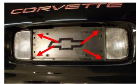
First remove the license plate. Behind the plate you will find four #15 torx screws. Remove all 4 to gain access to the reverse lights.
