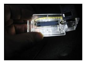
Un-hook the 2 wire loops from the end on the factory bulbs. (careful, they may still be hot). Remove the bulbs. Install the new led bulbs and test. Led bulbs are polarity sensitive so if they don't light, swap ends and re-test. Be sure to face the leds toward the clear lens and not toward the metal shield. Make sure interior lights havent timed out which they may do after about 15 minutes. You may need to adjust the metal arms to secure the leds.
