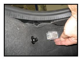
Remove the rear compartment lamps from the carpet.
