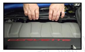
Start by pulling up on the coil covers as shown. They simply pull up. Then slide them up and out.
