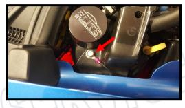
On ZO6 or Z51 cars you can use the 10mm bolt on top of the oil tank for a good ground.
