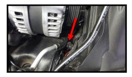
For ground connection look for a ground stud below and in front of the alternator on the frame. Hide the ground wire best you can under existing piping then secure with supplied nut. See next picture for ground option on Z-51 or ZO6 cars.
