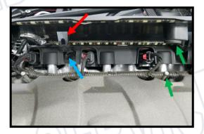
To install the covers you must line up the hooks on the bottom edge of the cover (red arrow) with the openings on the engine (blue arrow). There are 2 of them. The grommets on the top of the cover must align with the studs on the engine (green arrows). You will have to lower the covers so they fit under the cowl then align all these points to press in place.
