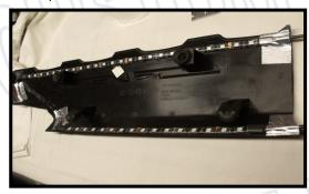
This shows how to mount the strips on the passenger side cover. Position the strips so the ends can be secured with the heat tape. Prep the mounting area's with alcohol then adhesion promoter. Come back after awhile and press the strips in place a final time.
