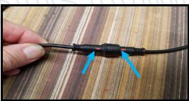
Connect the coil cover leads. Make sure you line up the arrows on the connectors and plug them in. Screw the plastic nuts to secure. Tuck these wires behind the cowl after installing the covers. The wires are a little long to aid in removing the covers. You can fashion them in a S pattern to hide them behind the cowl.
