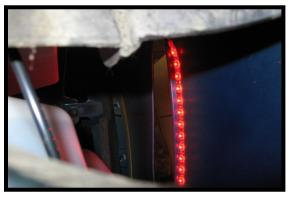
It helps to put a light in the cove area so you can find a path from above to route the led strips. The drivers side is easy. Just drop the leds past the W/S washer bottle into the cove area. Wipe the area around the opening with alcohol swabs. Best results are achieve by mounting the strips on the inside of the fender about an inch from the opening facing the cove shield
