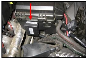
After all wires are secured and lights are working, You can now mount the control box on the fuse box or under the cowl lip above the battery. You can now reassemble all shields. Remember, the Inner fender panels have a hooked clip on the top that should go in first. Enjoy the new lights!!
