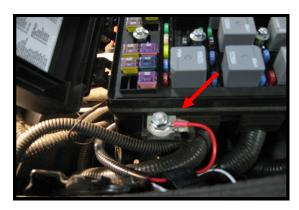
Open the cover over the positive battery connection at the under hood fuse box. Place red wire from control box over this stud and secure with provided nut. You can also connect it to the battery.
