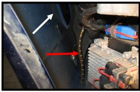
On the passenger side, Use a coat hangar to find a path down to the cove area (red arrow). Route leds down to the cove opening and use the same procedure to mount them as the drivers side. Mount on the inside of the fender facing the cove shield (white arrow). **IMPORTANT**; Use some very strong tape such as duct taper or gorilla tape to secure the wired end of the strip to the inner fender so it doesn't pull off.
