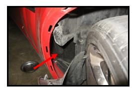
Shield removed to gain access to cove area. Leds will drop into this area for installation.
