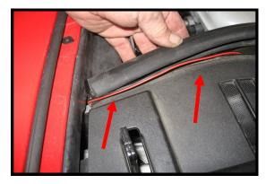
After leds are working you will need to hide the wires under the cowl weatherstrip or behind the engine away from the exhaust. You can tape the wires to the top of the cowl and slide the weatherstrip over being careful not to damage the wires.
