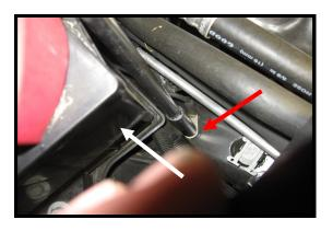
Below the battery tray (white arrow) along the frame rail there is a ground nut (red arrow). Place the black wire from the control box over this stud and attach with the provided nut. You can also connect it to the battery. You can now test the cove lights.
