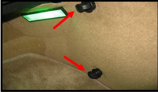
You can tap into the wires on either side. Decide which side you want to tap into and remove these 2 plastic cargo net nuts, remove the light housing to gain access to the wires.
