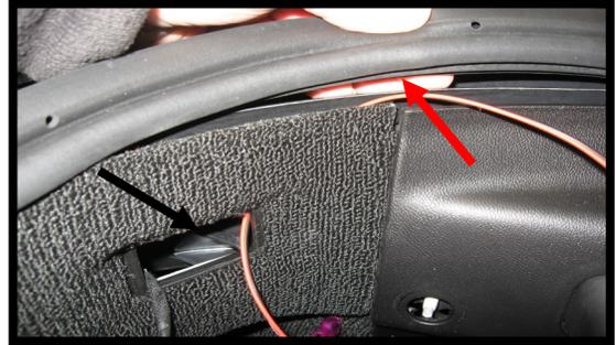
Pull up on the weather strip (red arrow) and pass the led wires through the opening ( black arrow).
