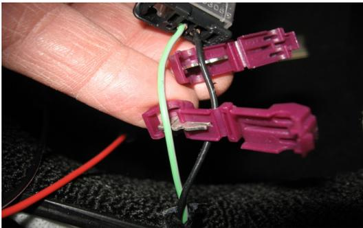
This illustrates how to use the connectors. Your wire colors will be different. (see next text box). Place the wires in the metal V and close with pliers until they latch.
