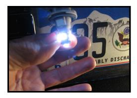
Turn on the lights. Plug in the led bulb. If it doesn't light, turn it 180 degrees and re-insert.
