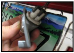
Remove the light housings, twist the grey socket 1/4 turn counterclockwise to remove it from the housing.
