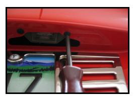
Using a #15 Torx screwdriver, remove the 2 screws holding the license light in place.
