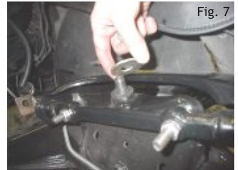
**NOTE:** Hand-tighten the nut ONLY. Do not compress the spring by tightening the nut on the stud. Wait until all of the suspension is installed and the car is back on its wheels before you finally tighten the nut.
