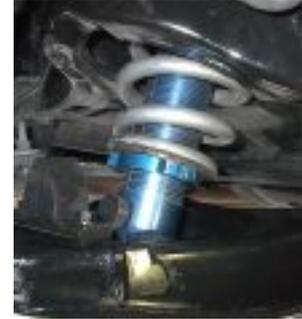
**PLEASE NOTE:** These shocks feature a small hydraulic bypass that allows them to be extended and compressed by hand. The actual shock valving does not begin to work until the velocities are higher than what can be applied by hand. Therefore, you will not be able to notice a change in stiffness when you change the valve settings and operate the shock by hand.
