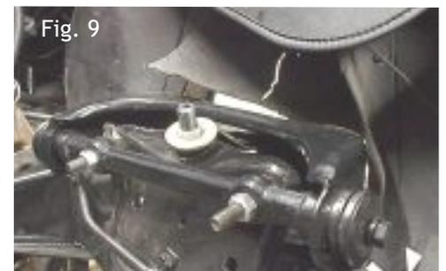
14. Tighten the top nut on the shock stud only after the weight of the car is on the wheels. Don't over-tighten (no more than 8 ft/lbs.) as the nut is aluminum and can easily strip. Check the tightness of the nut after the car has been driven for a few miles and the suspension has settled.
