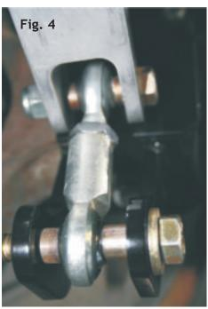
17. Place the other end of the shock in the center mount and install the 1/2"x2" bolt and nylock. Torque to 30 ft/lbs.
