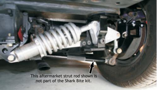
flat head bolts. **Tighten the support strut first and the cross member bolt last.** Torque 7/16" bolts to 50 ft/lbs and flat head bolts to 30 ft/lbs. Do not install strut backwards- see Page 3 diagram.
