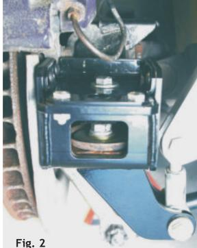
12. Place a 2" diameter washer inside the trailing arm cup. Slide the trailing arm mount onto the trailing arm and secure it with a 1/2"x1.5" bolt. Torque to 100 ft/lbs.
