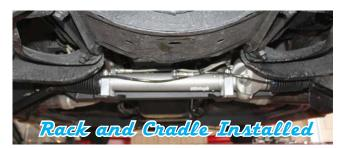
3) Install the OEM outer tie rod end into the Flaming River inner tie rod end on the new power rack. Note: If using the original parts some adjustment of the tie rod assembly may be required when connecting the to the spindle arm and the travel bar.
