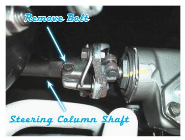
1) Remove the bolt that retains the rag joint coupler to the factory steering column shaft and spread flange.
