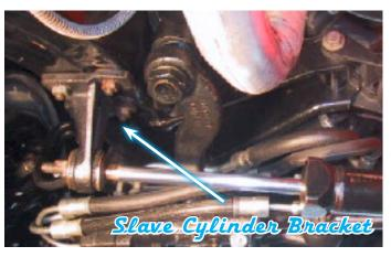
If your vehicle has power steering, remove the power steering lines from the pump to the power steering control valve and drain your system. Then, remove the four bolts that retain the power steering slave cylinder bracket to the frame rail. (If installing manual cradle, also remove power steering pump)
