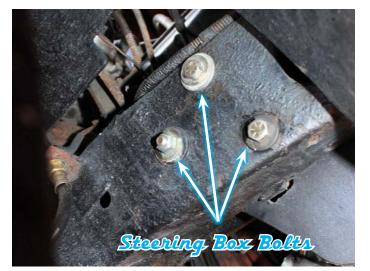
3) Remove the bolts that hold the steering box to the frame, and then remove the box from the car.
