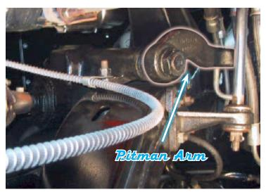
2) Remove the pitman arm from the steering box using a pitman arm puller.
