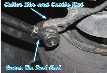
4) Next remove the bolts that hold the idler arm bracket to the frame and remove the cotter pins and castle nuts and separate the outer tie rod ends from the spindles.
