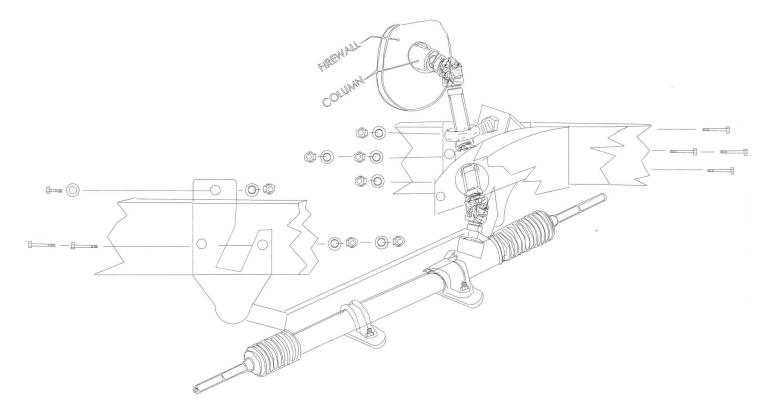
1) Begin by centering the rack. Turn the rack all the way to the left. Next, turn it all the way to the rightcounting the number of turns. Then go back to the left half the number of turns.
