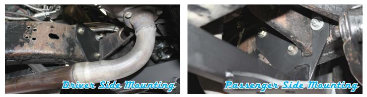
1) Install the rack and pinion cradle by sliding it into place between the frame rails. Using the new hardware, install the three (3) 3/8" bolts on the drivers side using the original holes from the steering gear box and the additional hole that is located under the factory motor mount. On the passenger side use idler arm bolts and the additional hole that is located under the factory motor mount (3) 3/8" bolts and tighten all the bolts and nuts to 40-45 ft. lbs.
