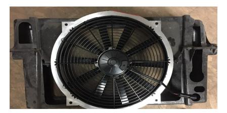
Step 4: Attach fan kit using the stock Bolts
