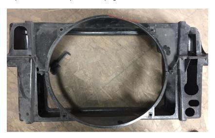
Step 3: Looking at the new SP464 fan kit, locate and align the same flat spot on the aluminum shroud to the flat spot on the stock shroud
