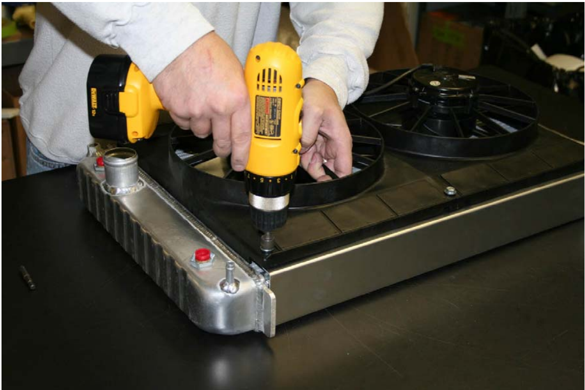
Step 4. While pulling up on the fans, snug the bolts tight with an electric drill motor.
