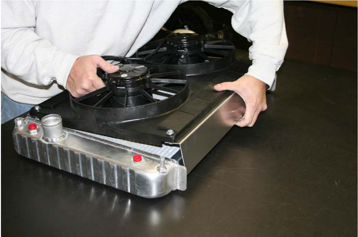
Step 3. Open top mounting bracket wide enough to slip over top of the radiator.
