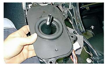
04: With the console top out of the way, you can now remove the four 10mm bolts on the rubber shift boot and lift the boot off.
