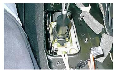
05: Then remove the four 10mm bolts at the base of the shifter and lift off. Use a razor blade to remove any old gasket material from the linkage-mounting base. Pop off the black plastic insulator on the bottom end of the stock shifter and install on your Kirban Kwik 6-speed Corvette shifter.
