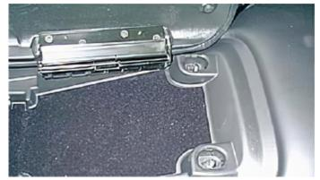
02: To remove your Corvette's center console, lift the center storage bin and locate the two plastic tabs at the rear of the bin. Lift off the plastic tabs to access the two 10mm nuts and remove them.
