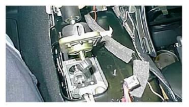
06: Apply a bead of silicone RTV to the base of the new Corvette shifter.
