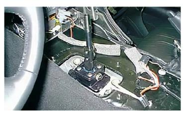
07: Install the new C5 Corvette shifter with the 4 supplied bolts and hand tighten. Once they are hand tightened, then torque the bolts to 20-25 ft.-lbs. in a cross pattern.
