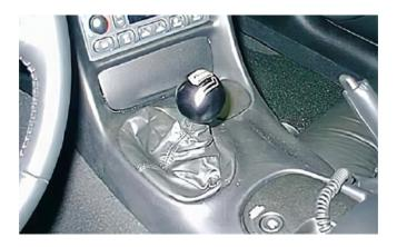
09: If you are keeping the factory shift knob, screw it on and replace the pressure pin. Use a soft mallet to drive in the pressure pin and you're ready to bang some gears!
