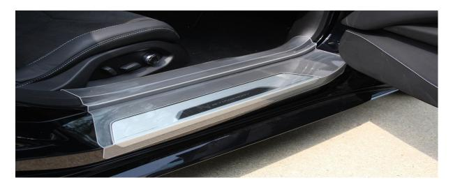
To install the Sill protector line the back edge up with the parting line on the plastic portion of the door sill. Hook the short edge on the painted portion of the door sill with hands on the Velcro gently pull sill protector over door sill. Be mindful of the front pillar as not to scuff during installation. Press the Velcro into the carpet.
