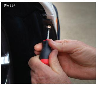
Now install the four (4) snap-head screw studs. Repeat this step on the other side of the car.
