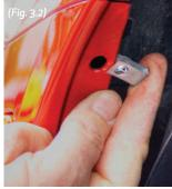
**Note:** the pin is a male/female assembly. The male piece can be pried loose from the female piece using a flat blade screwdriver. Insert the blade of the screwdriver in the slot at the edge of the pin and twist the screwdriver causing the pin to come free of the female piece. After removing the male piece, the female piece can be removed.
