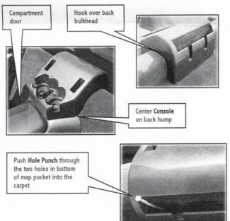
Remove the Console. Lift the back cargo area carpet and push the pointed tabs of the Fastening Panel through the punched holes as shown.
