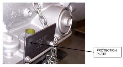
• INSTALL ISOLATOR MOUNT TO BOTTOM OF TRANSMISSION TAILHOUSING USING HARDWARE PACK HWG-PACK H.
