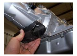
• NEVER INSTALL A SOLID ISOLATOR MOUNT – THIS COULD CAUSE CASE TO BREAK.
