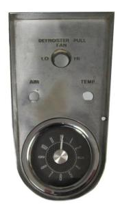
3. Reinstall the clock bezel in to the dash and refer to the Operation Manual to complete the clock setup.
