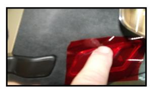
Work the tint into the edges of the lens around the front side of the lens first. Next move to the rear of the lens behind the button. Lift the tint while working it onto the lens behind and around the button. It tough to get the back of the lens covered without 1 small crease but where its at it doesn't show easily.
