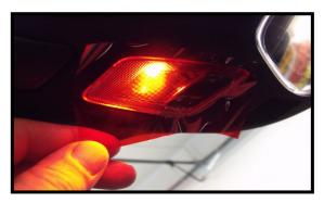
One extra sheet is provided in case you make mistakes. Remove the adhesive backing by placing a piece of scotch tape on each side then pull off the backing with the tape. Carefully lay the film over the light making sure the entire light is covered.
