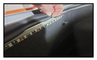
Pull the lip of the weather strip over the exposed portion of the led bar hiding the wire the best you can. Do this around the entire weather strip that you remove. That's it! Enjoy the new lights.
