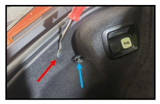
Remove the trunk net. Using the panel tool remove the flat retainer (red arrow). Unscrew the net retainer.
