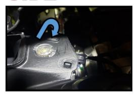
Force the light clockwise so it unlatches from the panel. Unplug the connector using the same method as the other side. You can put the factory light back in place or store it. Plug in the led strip. Keep in mind the lights may time out.
