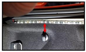
With the led strip with the connector end on the passenger side, slip the channel over the trunk liner aligning the slot on the back of the channel directly above the trunk net retainer. The channel is flexible so you can shape it to match the slight bend in the trunk.
