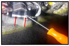
Release the factory light at the 2 points and pry the housing out.
