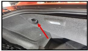
Remove the trunk net retainer on each side of the trunk to gain access to the factory lights.
