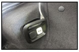
Pry out the light housing starting at this corner. The bracket that the light attaches to is very flexible so we found it is best to also push the housing out from behind at the same time. See next picture.
