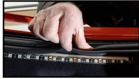
Install the weather strip u channel over the trunk outer liner while pulling the front lip of the weatherstrip out to cover the led channel bracket and inner liner.
