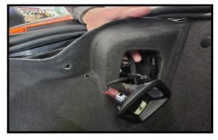
Pull back the trunk liner and push out the retainer clips and remove the light housing.
