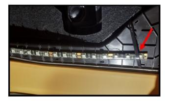
Prep the area along the 2 ribs with alcohol wipe and adhesion promotor. We like to slide the side toward the console under this tie strap and secure the rest of the strip along the ribs. Don't take the adhesive backing off the area that gets tucked under the tie strap or it will be difficult to slide the strip in place. Pull the adhesive backing off the rest of the strip and press it in place a couple times.
