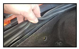
You can now re-install the weather strip. The uchannel on the weather strip goes over the rigid outer liner and the lip under my thumb will cover the inner liner.
