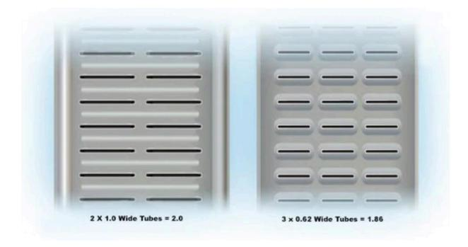
The U.S. standard for performance aluminum radiator tubes is a 1.0" wide tube and imported radiators have smaller 16mm (.62") tubes. In this case a 3-Row aluminum radiator would only have a total of 1.86" of tube-to-fin contact surface which is less than the two row core with 1" tubes.
