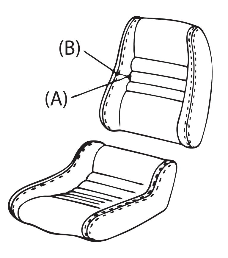
'78-82 seats came in two styles of side bolster. Using your original seat foam, determine pleat size by first locating end of horizontal pleats "(A)" on seat back insert. Then locate center point of double-stitching line "(B)". Measure distance between (A) and (B) – it will be either 2" or 4".
