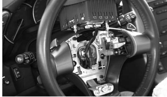
4. Using your T20 screw driver, remove the torx screw retaining the plastic cover on the wheel. This is the only screw that holds the cover; the other side has a tab that once you pull out on the cover it will come out. In order to install it later, insert the tab first and just push the cover into place and reinsert the screw.
