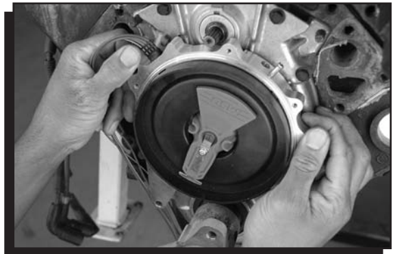
Figure 9 Installing the New Distributor.
