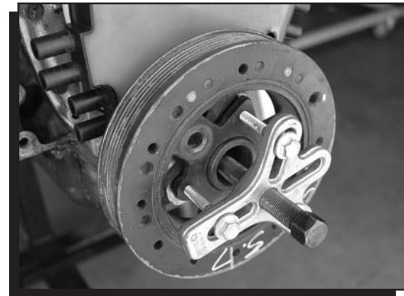
Figure 4 Removing the Hub.
