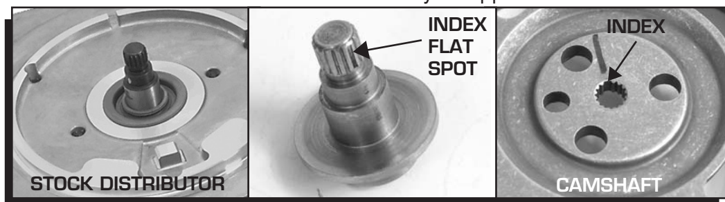
Figure 1 The Drive Mechanism of the PN 8381 Distributor.
