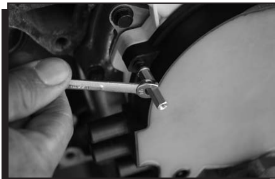
Figure 6 Removing the Original Cap.
