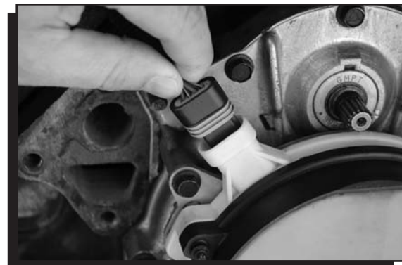
Figure 5 Disconnect the Distributor Connector.
