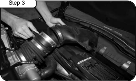
Lift up air box carefully from middle. Pull back MAF sensor from OE tube.
