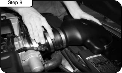
Install coupler to throttle body using clamps provided. Place tube to factory position and install completely. Do not tighten.
