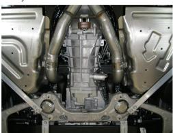
**Step 3.** Next, Loosely attach the Muffler Assemblies to the Inlet pipe using the provided 3.00" clamps. You will then need to fasten the provided cross bracket in place between the two muffler assembles using the provided 1/4" fasteners. Insert all hangers into the rubber isolators.
