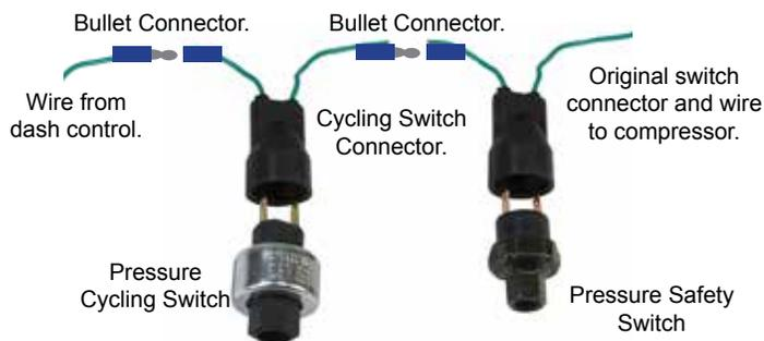
22) Clip wire between pressure safety switch and control and connect wires from pressure switch connector with bullet connectors as shown.
