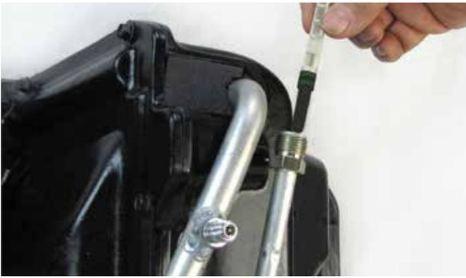
11) Insert Orifice Tube into Evaporator Inlet.
