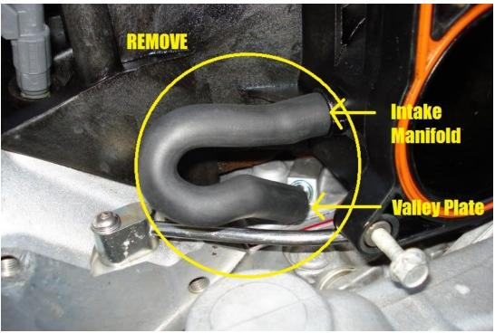
Connect can outlet to intake manifold factory PCV return port, Passenger side of intake manifold.
