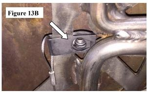
16. Install provided bolt and washer to Clip-On Nut. Torque bolt to 10 ft lbs. Secure Wire Rope Laynard path as shown. (See Figs. 14A & 14B)
