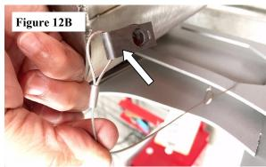
15. Slide Clip-On Nut to bracket on Right Side Muffler Assembly making sure it snaps into slot. (See Figs. 13A & 13B)
