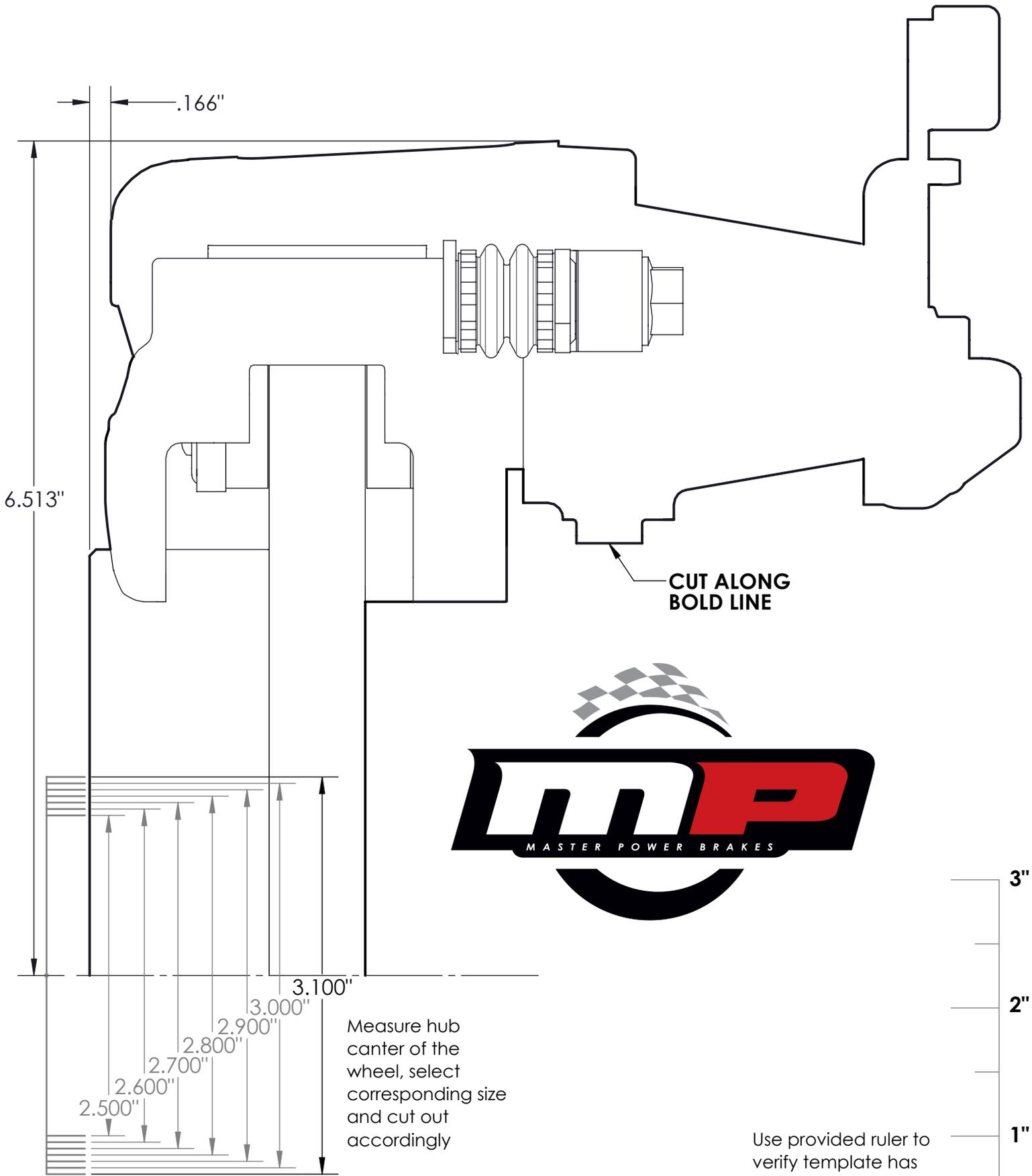
Measure hub center of the wheel, select corresponding size and cut out accordingly
