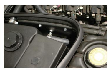
164. Reinstall the horn assembly by first plugging in the horn electrical connector and then attaching the horn bracket to the frame extension with its bolt using a 13mm socket and ratchet.
