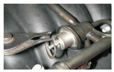
99. Using a small amount of oil or the supplied Lubriplate lubricant, lubricate the O-rings on the fuel regulator or pulse dampener and install into the new supplied fuel manifold. Reinstall the original C-clip using the C-clip pliers.
