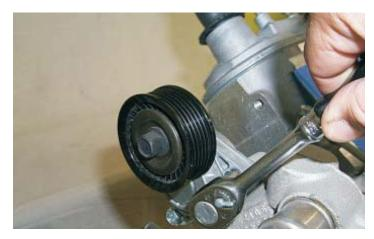
81. Install the stock idler pulley on the new tensioner assembly then install the assembly in place of the stock unit with the original bolts and torque them to 40 ft-lbs.
