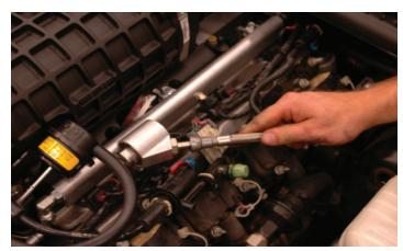
123. Re-install the fuel line safety clips. Test your connections!
