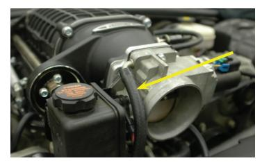
141. Using the supplied nylon wire ties, tie the throttle body coolant hose, TPS sensor wire, and the PCV breather hose together as shown.
