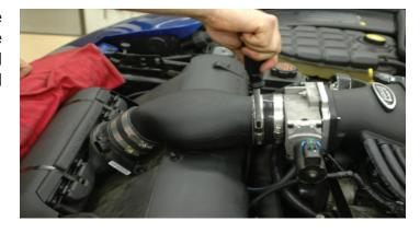
153. Connect the MAF plug to the MAF meter connection.
