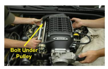
112. Remove any black plastic sleeves that hold the intake bolts up and start all ten intake bolts by hand, do not tighten until all the bolts are started. (Be careful not to cross thread the bolts.) Torque the supercharger manifold bolts, working from the center out in a crisscross pattern to 12 N-m (106 in-lbs) using a 10mm socket and a inch pound torque wrench.
