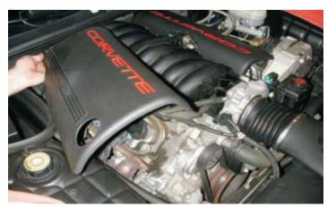
61. Remove the air cleaner duct from the throttle body and mass air flow meter (MAF). Unplug the intake air temp sensor (IAT) connector if applicable. Take care not to damage the meter, it is fragile. Some early model vehicles (97-01) will have the IAT sensor in the air cleaner duct. Later model vehicles (02-04) will have it as a part of the MAF sensor. The air cleaner duct will not be reused.
