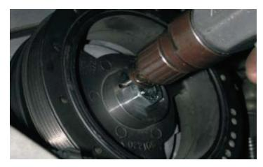
22. Using compressed air, blow the drill shavings out of the holes.
