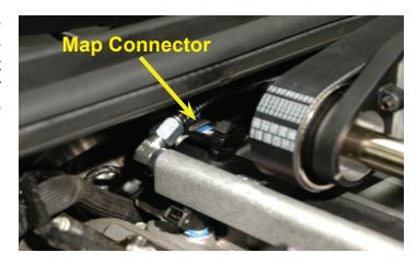
114. Pass the power steering hose through the fan belt as shown.
