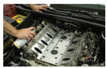
111. Carefully, with the help of an assistant, set the supercharger assembly on the engine. Line up the bolt holes with the holes in the cylinder heads. (Be careful of the one bolt that is under the rear supercharger pulley on the passenger side, as it hangs out a little and must be aligned first.)
