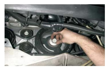
28. Using a 24mm socket tighten the new harmonic balancer bolt according to General Motors specifications. Tighten to 50 N-m (37 ft-lbs) then tighten an additional 140 degrees using a torque angle meter.
