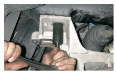
17. Using a pry bar, pry the cross member down on the driver side, until it stops against the nuts. Place a shim in the gap to hold it in this position. This clearance is needed to drill the crank for pinning.
