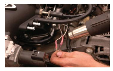
133. Install a new piece of the provided 1/4" split loom to cover the IAT harness back to the supercharger lid.
