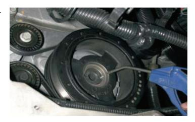
26. Insert the two supplied hardened roll pins into the drilled holes. The use of a small hammer and punch may be necessary to tap the pins in. (Make sure that the pins are in far enough that they do not touch the balancer bolt.)
