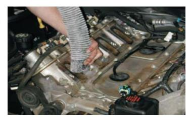
77. Cover the intake manifold ports with tape or clean rags to keep dirt and objects from entering the engine. (Remember, be clean.)
