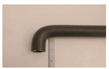
160. Attach one short hose end using the supplied worm gear clamps to the passenger side barb at the rear of the supercharger lid, route the hose over the fuel rail toward the passenger side and away from the supercharger pulleys, though your new notch in the battery partition, and connect to the hose barb on the intercooler reservoir using a provided worm gear clamp.
