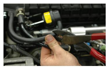
139. Trim the 1/4" vacuum hose that comes from the back of the driver side of the engine compartment to join with the remaining leg of the "T" connector. This is the hose that was installed in step # 110.
