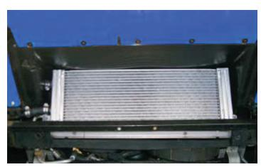
32. With the heat exchanger in position, use a pen or scribe to make a mark on the side of the radiator shroud to locate a new hole of at least 1" in diameter at the upper barb. Remove the heat exchanger and using a hole-saw or sharp knife make the hole in radiator shroud for the heat exchanger barb.
