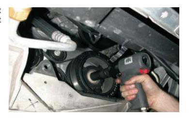
20. Install the drill guide using the supplied bolt and tighten to 30 ft-lbs with a 24mm socket and torque wrench.
