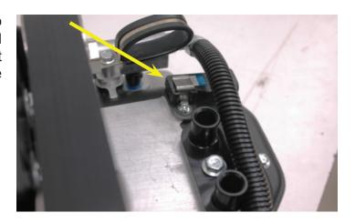
98. Using a pair of C-clip pliers, remove the stock fuel pressure regulator or pulse dampener from the stock fuel rail assembly on the stock intake manifold.
