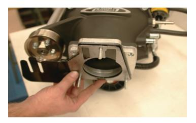
105. Install the throttle body on the supercharger inlet using the supplied hardware on the supplied mounting studs, sandwiching the power steering reservoir bracket from the previous steps. Torque the nuts to 12 N-m (106 in-lbs).
