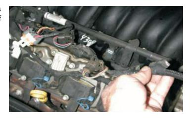
70. Disconnect the power brake booster vacuum line at the power brake booster by pulling the check valve out of the grommet.
