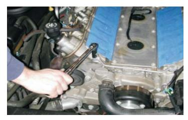
89. On the engine valley cover, remove the two black rubber knock sensor covers by gently prying them up using a small straight blade screwdriver. Disconnect the electrical connectors by squeezing the side of plugs with a pair of long jaw or needle nose pliers and pulling up.
