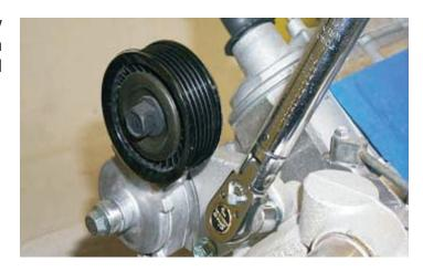
82. Using a 15mm socket wrench, remove the two 10mm bolts that hold on the power steering oil reservoir to the cylinder head. Remove the bracket from the reservoir and reinstall the bolts back into the cylinder head and tighten to 50 N-m (37 ft-lbs).
