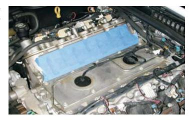
78. Using a 10mm socket wrench, remove the two or four coolant vent pipe bolts. (Some models have a small pipe in the front and some have a large pipe that goes from the front to the back.) Only remove the front pipe.
