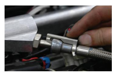
124. Connect the extended piece of 5/8" hose connected to the coupling in step #88 to the power steering reservoir tank using the supplied hose clamp.
