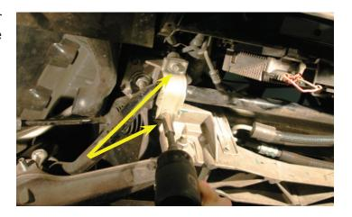
9. After removing the sway bolts, brackets and end link nuts, remove the sway bar and set it aside.
