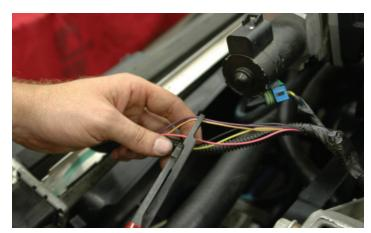
131. Locate and route the two white wires exiting from the middle of the driver side supercharger manifold lid forward, and verify that about 3/8" of wire are exposed. Use the supplied crimp connector to connect the tan and purple wires to the white wires, it doesn't matter which wire you crimp to which white wire.
