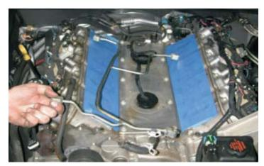
79. Remove the accessory serpentine belt by rotating the tensioner pulley bolt clockwise with a 15mm fan belt tensioner wrench. The belt will not be reused.
