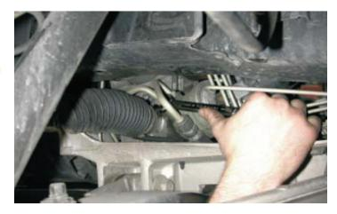
12. Remove the two bolts from the power steering cooler using a 10mm wrench. Let the cooler hang down out of the way.
