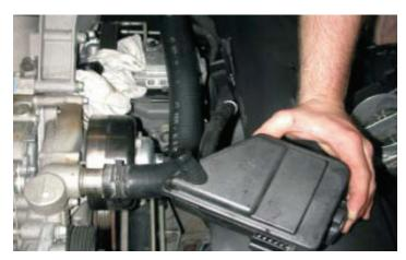
87. Using the stock bolts removed earlier, install the new front coolant vent pipe and rear block off blocks. (Late model vehicles already have the rear blocks installed.) Make sure that the small Oring gaskets are in place.
