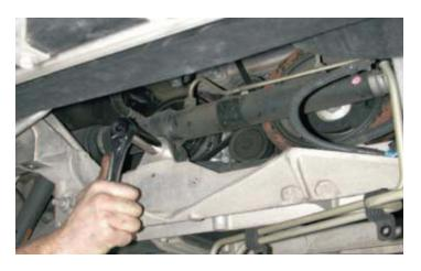
14. Remove the four bolts holding the ABS bracket to the frame with a 13mm socket wrench.
