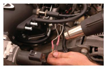
129. 2002-2004 Corvettes have the IAT sensor built into the MAF sensor: Pull back the split loom from the MAF sensor harness and remove the tape to expose the five wires.
