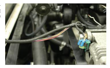
130. Cut the tan and purple wires about 4" from the throttle body connection split. Strip about 3/8" from the rear section of the cut ends of the tan and purple wires. The forward pieces can be covered with tape and pushed back into the remaining harness.
