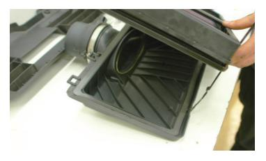
152. Install the new air duct from the throttle body to the MAF meter. Make sure that there are no air leaks. (On early models there is a small vacuum hose that goes from the duct to the fuel regulator nipple.)
