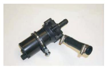
44. Pull the loose edge of the nose cover down so you can install the pump on top of the frame extension with the electrical connection pointing forward towards the front of the car. Slide the pump outlet hose on to the lower barb of the heat exchanger and secure it with a #10 clamp. The mounting clamp tabs should be pointing towards the center of the car.
