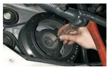
27. Install the new supplied factory GM harmonic balancer bolt.
