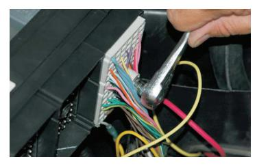
58. Remove the nut from the B+ terminal on the fuse relay center with a ratchet and deep 13mm socket. Place the ring connector of the larger red wire from intercooler harness on the B+ terminal and reinstall the nut securely. Replace the Fuse/Relay center and B+ covers.
