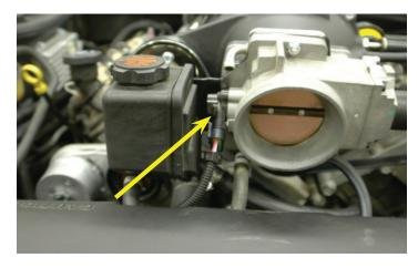
137. Connect the Electronic Throttle control connector.
