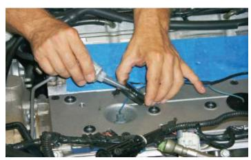
95. Remove the existing tape from the knock sensor wires so that they can be installed on the grooves in the top of the new valley cover. Use some tape to hold the wires in place temporarily, and then use some of the silicone adhesive to retain the wires permanently.
