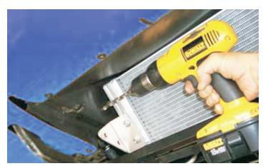
36. Replace the heat exchanger after drilling the mounting holes. Using the 8x25mm bolts and flange nuts supplied, bolt the heat exchanger in place on the left side only. Loosen the mounting bracket nuts on the right side only and temporarily slide the bracket down so that you can install the heat exchanger hose and #10 clamp on the upper barb.
