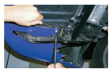
47. To ensure proper airflow to the heat exchanger, modify the center section of the front spoiler. From the backside using the mounting bracket as a guide, cut the upper rubber portion off along the top edge of the mounting bracket. Reinstall the front spoiler with its two aluminum center supports and four mounting bolts with a ratchet and 10mm socket.
