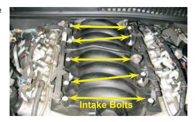
74. At the rear of the intake manifold, disconnect the MAP sensor electrical connector and vacuum line. (Be careful not to break the intake manifold as it is plastic.)
