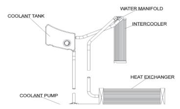
156. Temporarily position the intercooler reservoir on top of the battery and remove the rubber strip along the top edge of the surrounding partition. Using a pair of Tin-snips, mark and cut a notch in the top edge of the partition so that a hose can pass through to the upper barb of the reservoir. Reattach the rubber seal along the top of the partition.
