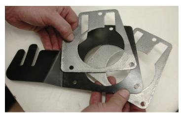
104. Screw in the supplied throttle body mounting studs into the three holes of the adapter plate and mount the power steering reservoir bracket to the throttle body location by placing a new intake gasket on both sides of the power steering reservoir bracket as shown.
