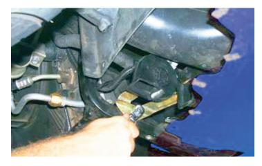
165. Reinstall the splash panel and corner of the spoiler to the underside of the nose with their eight mounting bolts, using a 7mm socket and ratchet.
