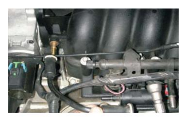
64. Disconnect the electrical connectors from the throttle body, TPS, ETC and also remove the crankcase PCV vent hose.
