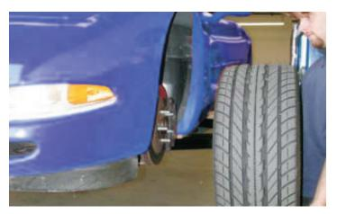
6. Remove the right and left outer tie rod ends from the steering knuckles using an 18mm wrench and a 6mm Allen socket wrench.
