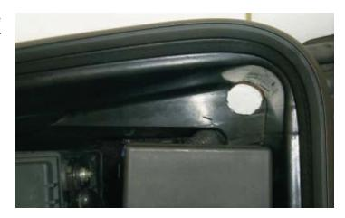
158. Using the Peel-and-stick pad supplied, attach it to the side of the hood latch next to the battery. This will act as a cushion for the reservoir.
