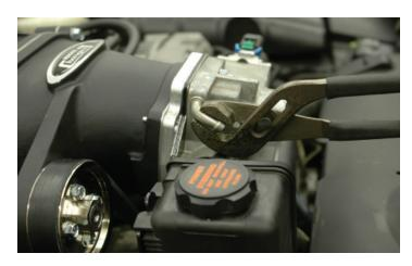
136. Reconnect the throttle body electrical Throttle position sensor connector.
