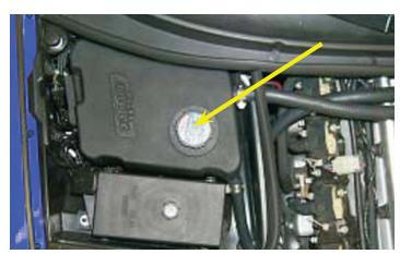
167. Close the radiator petcock and reinstall the coolant saved from step 4. If more coolant is needed, only use coolant recommended by GM.
