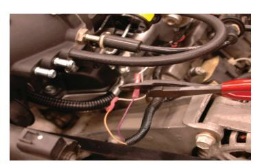
128. Heat-shrink your connections using a hair dryer on high or heat gun. It is not adequate to just crimp the connections together. Recover the wires all the way to the lid using the original split loom and any additional length of the provided 1/4" split loom necessary.
