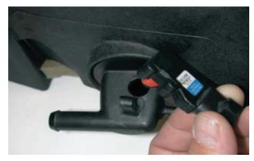
97. Use the provided Lubriplate lubricant to lube the O-ring, then install the MAP sensor and seal on the supercharger manifold by pressing it in the hole and using the supplied bracket and the short 6mm button head Allen bolt.
