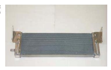
34. The brackets attach to the heat exchanger by sliding into the open ends of the channel on the front face of the heat exchanger side tanks. The square portion of the bolt shaft must be aligned with the side channel. Tighten the mounting nuts to lock the brackets in position.
