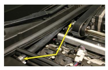
161. Attach the other short hose end using a supplied worm gear clamp to the driver side barb at the rear of the supercharger lid. Route this hose parallel to the other hose, toward the passenger side fender, forward and cut to join the coupling (hose-mender) on the hose from the top barb of the intercooler heat exchanger you connected in step #50. Secure using the provided spring clamp.
