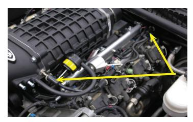
119. On the driver side rear of the supercharger manifold, locate the pressure port capped with a small, rubber cap and remove the cap. Using the hose supplied, connect one end of the hose to the pressure port and then route the other end to the Fuel Pump Booster module. Secure the hose out of the way of the rotating parts at the rear of the blower with the Ty-wraps supplied.
