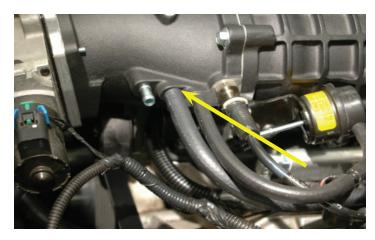
148. All vehicles continue from here: Install the check valve on the 11/32" vacuum hose and plug the check valve into the grommet on the brake booster.
