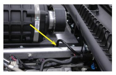
120. Connect the remaining end of the hose to the Fuel Pump Booster vacuum barb. Secure the hose out of the way with the Ty-wraps supplied.
