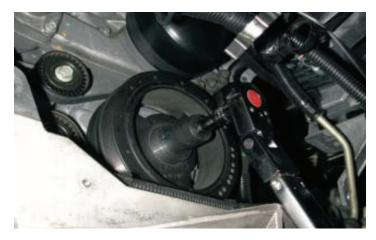
21. Using a small or angled 3/8" drill and the supplied drill bit, insert the drill into the guide holes and drill to the second step of the drill bit. (Make sure that you drill all the way to the second step.) We recommend safety glasses during all steps. Please be sure to wear them during these steps.
