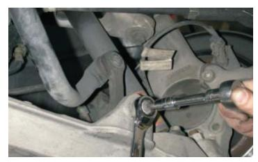
8. From under the vehicle, remove the four bolts that secure the sway bar brackets to the chassis with a 13mm socket wrench.
