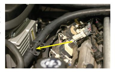
162. Install the Adel clamp to secure the two intercooler hoses (removed earlier from the passenger side fuel rail, rear mounting bolt when you were working with the MAP sensor), incorporate the spacer removed at the same time.
