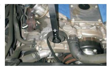
80. Remove the stock tensioner assembly by removing the two mounting bolts with a 15mm wrench. You will need to remove the stock idler pulley as well. It's easier to remove the pulley first.
