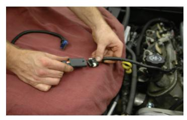
135. Using a pair of pliers carefully turn the PCV vent tube to the forward position as shown in the picture.
