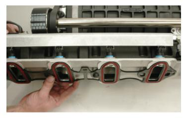
109. Remove the protective tape from the cylinder heads and supercharger. Clean off any tape residue using alcohol or some other non-petroleum based solvent. IMPORTANT: Make sure that there is no debris in the ports.
