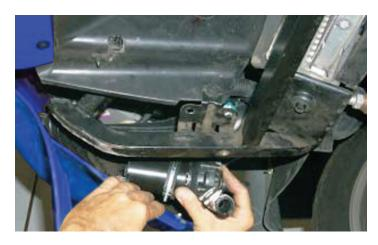
45. Here is a view from the other side of the pump installed with the outside edge of the nose cover pulled back. The pump will be mounted by passing the mounting clamp bolt through the hole in the frame extension tab (where you previously removed the clip nut). Then through the nose cover flap to be secured with the nut and washer on the bottom of the car.
