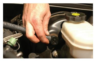
149. Route the hose forward and plug into the remaining hose barb on the supercharger inlet.
