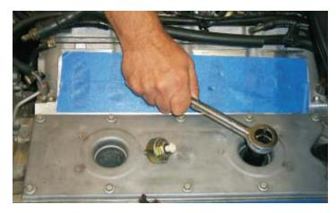
91. Remove the engine valley cover and gasket by removing the ten bolts with a ratchet and 10mm socket.
