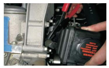
85. Using the supplied 5/8" hose mender and 5/8" hose clamp, install the power steering reservoir hose to the power steering pump.
