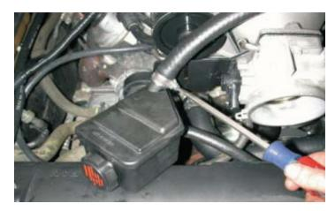
125. Install the power steering reservoir on the reservoir bracket.
