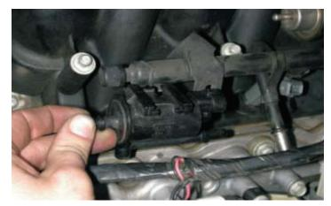
69. Disconnect the fuel injector wire harness from the clips and lay the wiring aside and out of the way.
