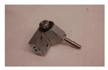
100. Lubricate the supplied O-ring with the supplied Lubriplate lubricant and install into the driver side fuel rail manifold recess as shown.
