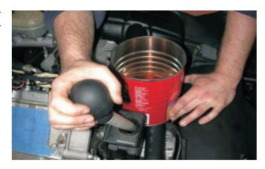
84. Using a pair of hose clamp pliers, remove the large hose clamp on the power steering reservoir and remove the reservoir from the hose. Place a rag under the reservoir to catch any oil dripping.
