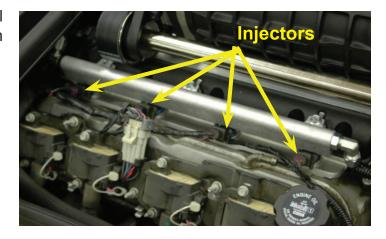
122. Push the stock fuel lines (one or two) onto the new fuel manifold fittings. Make sure that they are locked on by pushing and pulling on them lightly.
