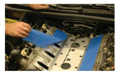
110. Spray silicone or some mild soap and water solution on the cylinder head surface to lubricate. This makes the intake manifold slide around a little to help line up the holes. (Do not use anything that will damage the intake gaskets, petroleum based products, etc.)
