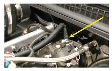
146. Route the hose forward, below the fuel rail manifold, cut to fit and connect the remaining hose end to the 3/8" hose barb located on the supercharger inlet as shown.
