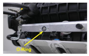
101. Mount the new fuel supply manifold to the driver side fuel rail using the supplied bolts and torque to 106" lbs. Ensure that the O-ring remains seated correctly and doesn't get pinched over the edges.
