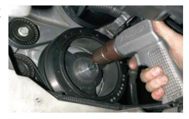
24. Using a 24mm socket, remove the large bolt and the drill guide from the engine.
