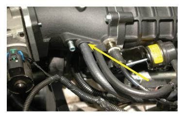
147. For non Z-06 models: Cut a section of the provided PCV hose to run from the hose barb located on the rear of the driver side valve cover, route forward, below the fuel rail manifold and connect to the hose barb on the supercharger inlet.
