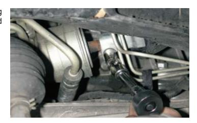
11. Using an 18mm line wrench, disconnect the power steering high and low pressure lines from the rack and pinion. Use a drain pan to catch any fluid. Be careful not to damage the seals on the end of the lines.
