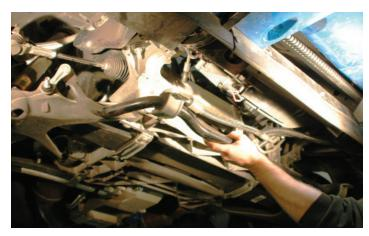
The crank pulley needs to be pinned to avoid spinning. This entails having the clearance necessary to get drill motors in front of the crank pulley. The way to get additional clearance is to remove the Rack and pinion steering assembly, this is covered in the next eight steps:
