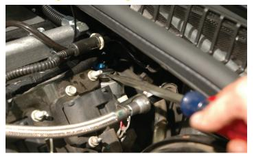
144. Assemble the final PCV hose by cutting a 2" length and attaching one end to the 90° "Elbow" fitting. Attach the other end to the new PVC valve. From the remaining hose cut a 38" section and connect one end to the remaining barb on the elbow fitting.
