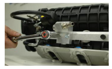
102. Using a 10mm socket wrench remove the throttle body from the stock intake manifold.
