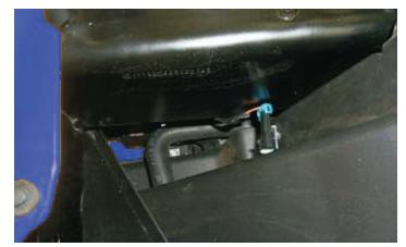
38. Here is the heat exchanger bolted in position with the hoses installed.
