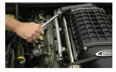
113. There is an Adel clamp at the rear passenger side fuel rail mounting bolt with an incorporated spacer. Remove this assembly and set aside for later re-install. Plug in the (MAP) sensor electrical connector at the rear of the supercharger manifold.
