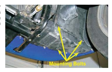
41. After removing the right hand splash panel, remove the horn assembly by unbolting its mounting bracket with a ratchet and 13mm socket. Pull the assembly free then disconnect its electrical connection.
