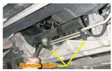
13. Remove the two large bolts holding the rack and pinion in place using an 18mm socket wrench and an 18mm wrench.
