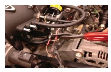
132. Use a hair dryer on high or a heat gun to shrink your connections. It is not adequate to just crimp the wires together. This also helps avoid moisture contamination.
