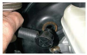
71. Remove the knock sensor wire harness connector from the PCV tube and unplug.
