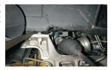
18. Remove the rack and pinion from the vehicle by sliding it out the driver side
