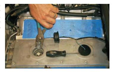
90. Remove the two knock sensors by using a ratchet and a deep 22mm socket.
