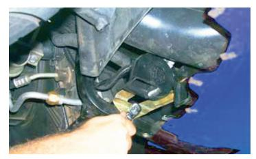
42. On the inside of the frame extension tab, remove the bolt and clip nut that secures the inner flap of nose cover with a ratchet and 7mm socket. Pull the nose cover flap down and out.
