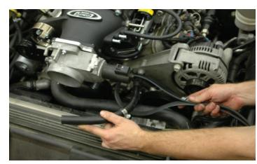
115. Install the new supplied supercharger and accessory fan belt with a 15mm tensioner wrench, using the new supplied belt routing diagram below.
