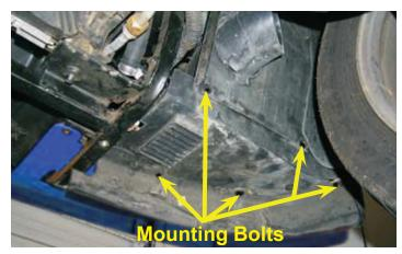
40. Remove the right hand splash panel by removing the two mounting bolts and washers on the bottom surface and the two along the bottom edge of the wheel well with a ratchet and 7mm socket.
