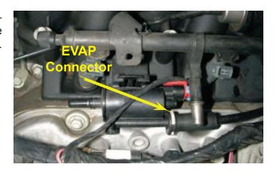
68. Remove the EVAP canister solenoid and mounting bracket.
