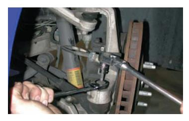
7. Remove the nuts that secure the sway bar end links to the lower A-arms on both sides of the vehicle. Use a T-40 or 6mm socket (depending on the year) and an 18mm open-end wrench.
