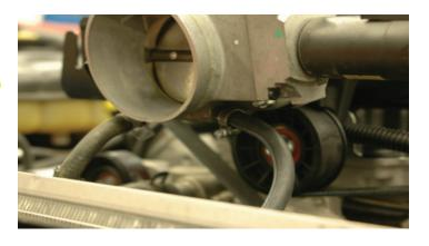
118. Assemble the EVAP Sensor and hoses as original and install the EVAP hard line connector onto the EVAP fitting located on the driver sided of the supercharger inlet manifold by pushing it on firmly. Route the other end back to the firewall hard-line EVAP hose barb located behind the driver side head and plug in securely.
