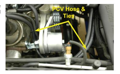
142. Connect the other end of the PCV hose from the throttle body to the passenger side valve cover barb as shown.
