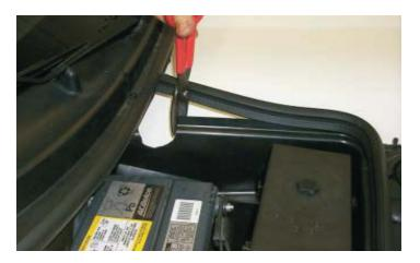
157. In the lower corner just ahead of the fuse relay center, create a hole, at least 1" in diameter on the partition floor so a hose can pass through to the lower barb of the reservoir.
