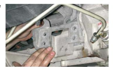
16. Using hand tools only, loosen, but do not remove the four cross member mounting nuts using a 21mm socket wrench. A breaker bar may be needed. Only loosen the nuts until the last thread is visible.
