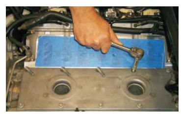
92. The gasket will be reused, the original valley cover and bolts will not. Inspect the gasket for any damage and then reinstall. Note: It will only fit correctly in one position.
