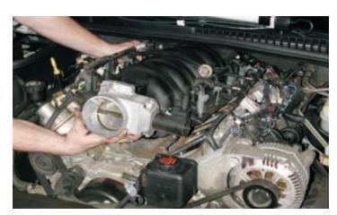
76. Using a vacuum cleaner, remove any dirt or debris from the intake port area. (Be careful not to get any dirt in the intake ports.)
