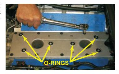
94. Reinstall the knock sensors and torque them to 15 ft-lbs. Reattach the electrical connectors by pushing the plug down firmly until a "click" is heard. Before installing the covers, apply a bead of the silicone adhesive supplied to the side of each of the covers. Finally push the covers back into place.
