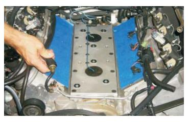
108. Install the new supplied intake gaskets (2) into the recesses in the intake manifold.
