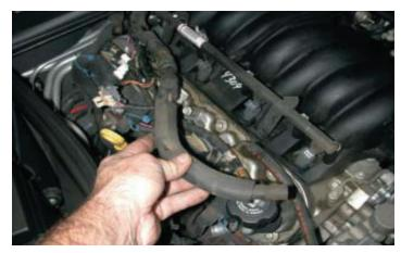
73. With a 8mm socket wrench remove the ten intake manifold bolts.
