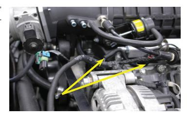
134. All vehicles continue from here: Connect the TPS sensor connector into the female end of the TPS extension supplied.
