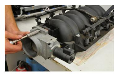
103. The supplied throttle body gaskets sandwich the power steering reservoir mounting bracket. Note the "UP" designations on the gaskets and verify that the idle slot is not being blocked by gasket material.
