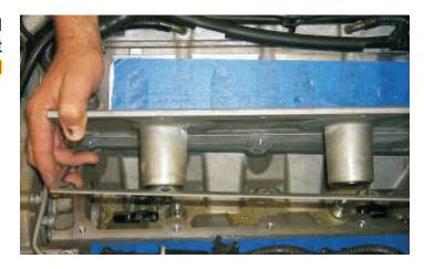
93. Install the new engine valley cover and flathead bolts supplied with a 5mm Allen socket and torque the bolts to 18 ft-lbs. Insert the six Orings in the recesses in the new valley cover.
