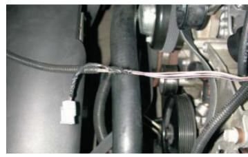
127. Expose about 3/8" of all wire ends and use the provided crimp-shrink connectors to join the wires together.
