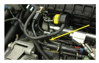
140. Install a 36" piece of 3/8" PCV breather hose to the throttle body barb. Route the hose toward the passenger side, down and back below the tensioner mounting bracket and up, over the valve cover and back paralleling the TPS sensor wire and throttle body coolant hose.
