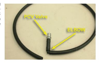
145. Plug the PCV valve into the hole created when you removed the plastic plug from the rubber grommet at the rear of the driver side valve cover.
