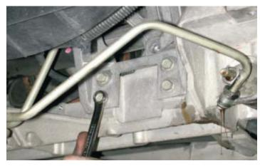
15. Push the ABS bracket up and out of the way.
