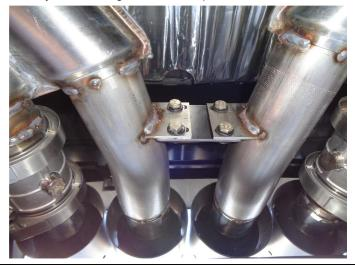
**Step 8.** Locate both OEM hanger brackets to each Tail Pipe Assembly. Next, loosely attach both assemblies to the Inlet Pipe Assembly outlets using the supplied 3.00" clamps. Using the supplied nuts, bolts and washers connect the two hanger brackets that will link both sides together. Reconnect each wiring harness connector the the valve motors. Reinstall the rear valence in the reverse order of the removal process.
