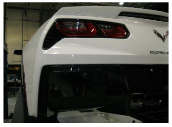
**Step 3.** Next, remove the six 10mm bolts from the valence top. Carefully release the tabs on the top of the valence. The valence may now be removed.
