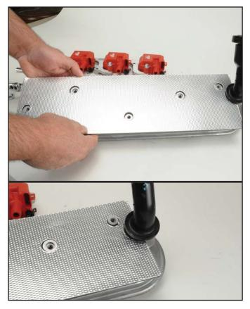
STEP 4. Depending on your application you may have to remove the plug wires from the spark plugs to give enough room to install the heat shield. **FIG 3**
