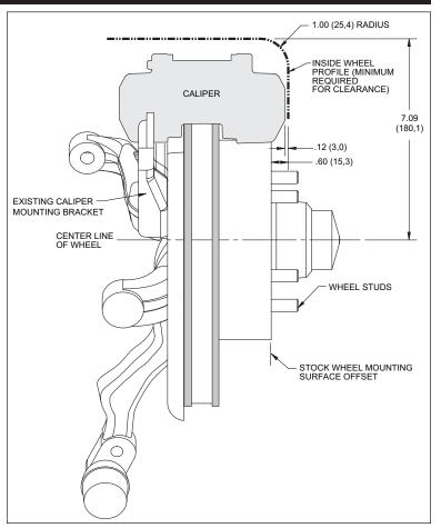
Figure 2. Wheel Clearance Diagram
