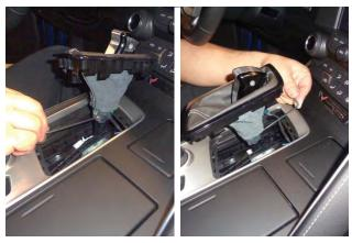
13. Tighten the set screws. (Pull the shifter back to reach the front screw, if required.)
