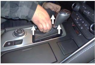
4. Carefully feel through the boot, and lift the bezel out of the center console.
