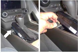
5. At the front driver side of the bezel, disconnect the electrical plug.
